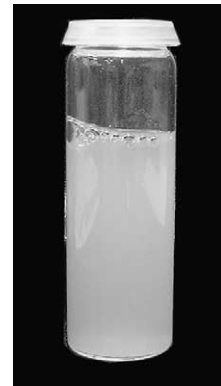
Fig. 6. Spray-dried microcrystals, dispersed in water (after 28 days).
